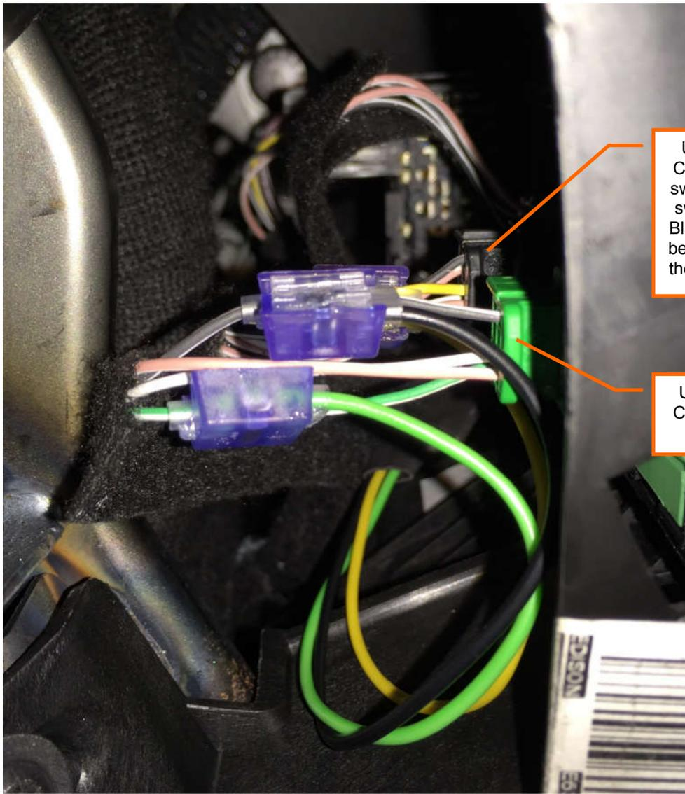
Unplug the Black Connector from the switch. If there is no switch present, the Black Connector will be in the area where the switch would be.
